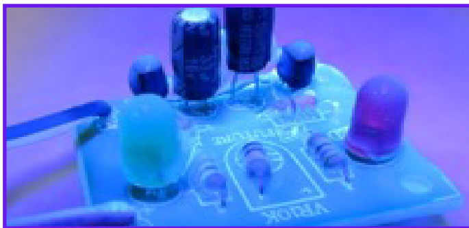
Figure 8. Conformal coated PCB assembly under UV detection light
