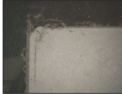
Parylene-Coated Tin Plated Brass Coupon
