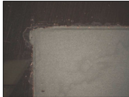
Parylene-Coated Tin Plated Copper Coupon
