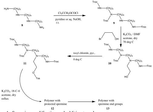
Scheme 4. Spermine modification and addition to polymer.
