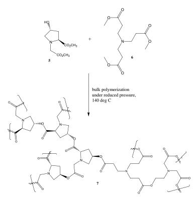
Scheme 3. Polymerization of N-(carboxymethyl)-trans-4-hydroxy-L-proline dimethyl ester.
