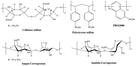
Figure 1. Microbicidal anionic ionomers.
