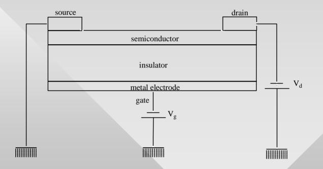
Schematic of the TFT structure used in an Organic FET.
