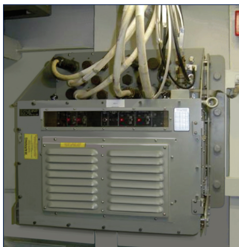
Figure 1-2: AN/USQ-82(V) IOU installed on Arleigh Burke-class DDG (Courtesy of The Boeing Company).
