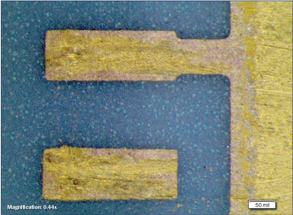
Figure 2-4: Detail of wire bond pad after cleaning
