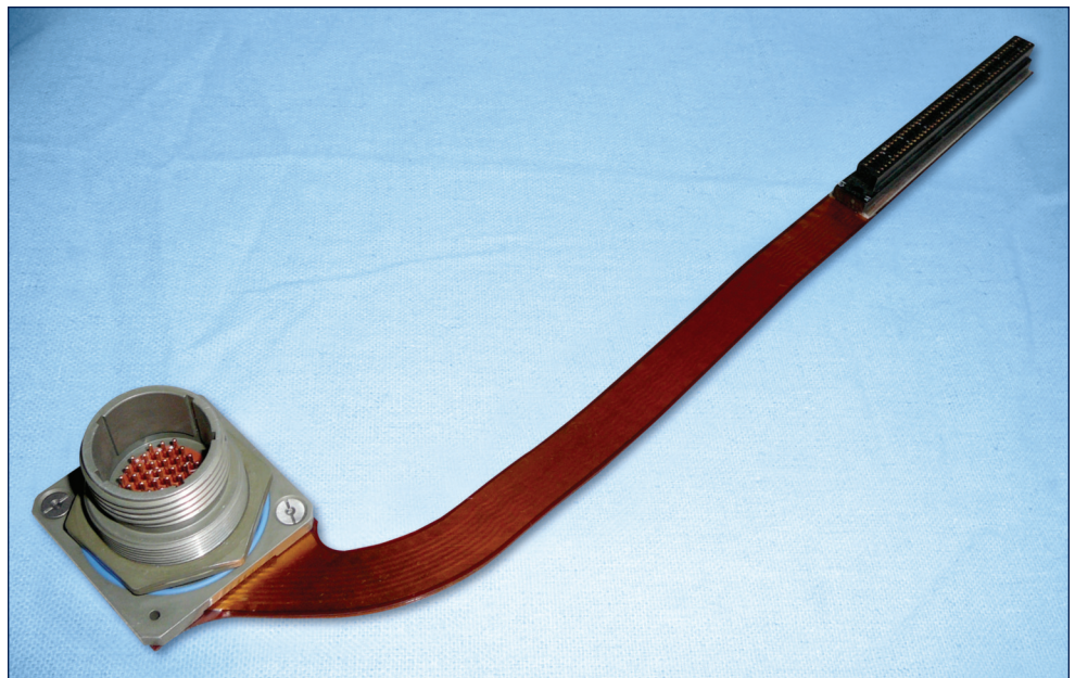
Figure 1-3: One of the flexible circuits in AN/USQ-82(V) IOU that will be redesigned to achieve gigabit Ethernet speeds (Courtesy of The Boeing Company).
